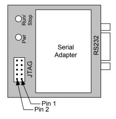
Figure 4. Serial Adapter JTAG/DEBUG Connector
