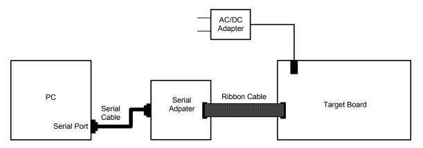
Figure 1. Hardware Setup
