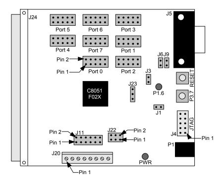
Figure 2. C8051F020 Target Board
